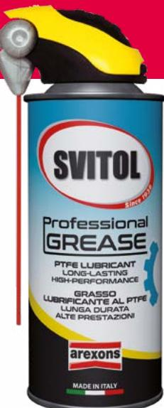
🇬🇧 A grease made up of mineral oil and aluminium complex soap with PTFE [polytetrafluoroethylene] and anti-friction additives. It provides long-lasting lubrication for mechanisms, bearings and gears and is suitable for use with rubber and plastic. High temperature resistance: -40 ° C to + 170 ° C, dew point 250 ° C.
